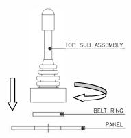
4. Tighten the lock screws in clockwise direction with a torque of 1.2Nm (max)
