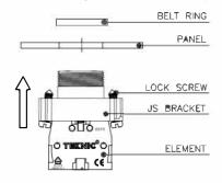
3. Ensure the belt ring is assembled from above the panel. Fully tighten the top sub assembly by rotating clockwise
